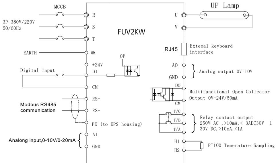
Note: "⊙" Main circuit terminals, "○" Control circuit terminals
